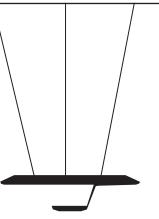
**EN** Hanging light with many lighting configurations, designed for large spaces and designed as a light machine to offer different lighting effects. A large disk with high visual impact and high reflector levels for direct and focused lighting. Lamps for indirect or reflected lighting, can be housed in the overhanging ring below.
