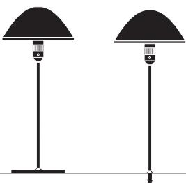
**EN** Classically elegant table lamp with aluminium base and stem. The diffuser, in opal blown glass, is supported by an arm extending out from the lampholder ring, whose cylindrical shape makes an easier assembly and disassembly of components.
